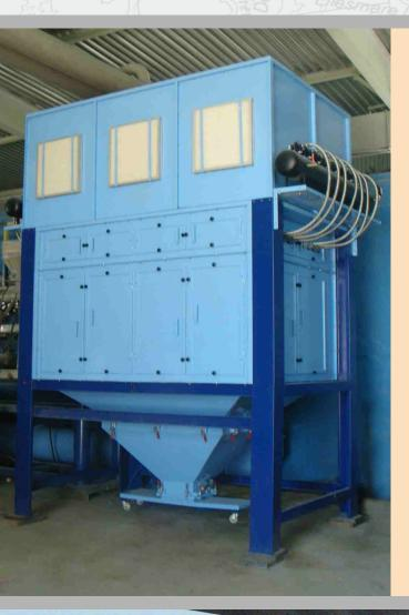
Cyclone, Rotary Cyclone recoveries will capture up to 98% of the overspray powder. The balance powder which is fine powder will escape out to the atmosphere. The cartridge type after filter will capture the fine powder and will only allow the clean air out.
